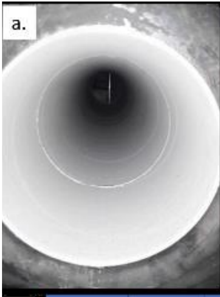
Pipe inner surface with Zn-Cr top-coat
