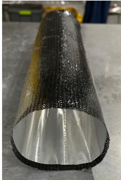
Resin-infused biaxial carbon fiber composite layer
